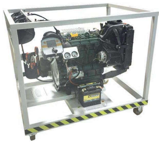
The Biodiesel Running Engine is designed for use in alternative fuels and technical education programs. It operates on B100 Biofuel and Diesel Fuel. This new agricultural engine demonstrates the use of biofuels from many sources.
