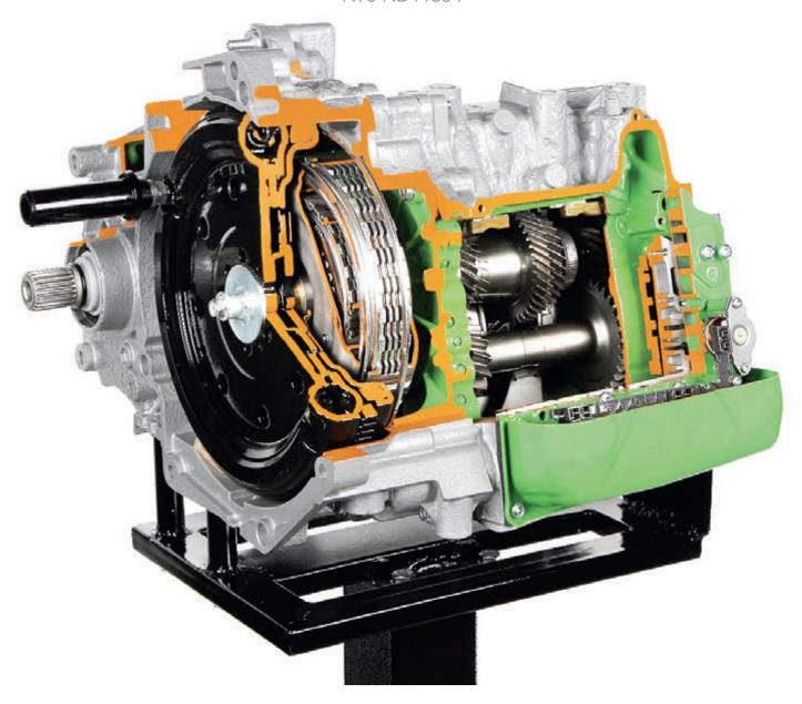
The Direct-Shift Gearbox (also referred to as double-clutch gearbox) has two main shafts; one for the odd gears and the other for the even gears. Each shaft is inserted into one of the discs of the coaxial clutches. The shafts connected to the clutches can transmit motion mechanically to an auxiliary shaft having the relevant speed-gears.
