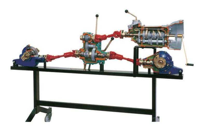
Transmission assembly fitted to most 4x4 cross-country vehicles. The various parts are provided as accurate cut-away models, connected together to show their operation in an easy, immediately understandable manner.
