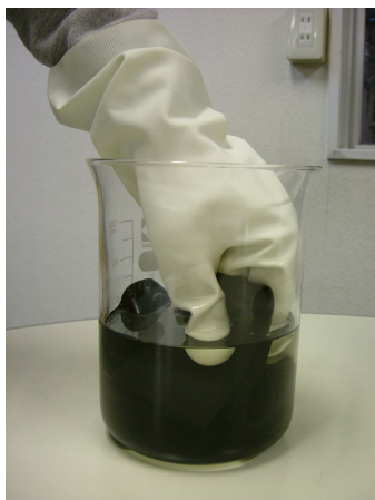
Fig. 13 Cleaning the Belt in a 1-liter Beaker Filled with Ethanol for Disinfection
