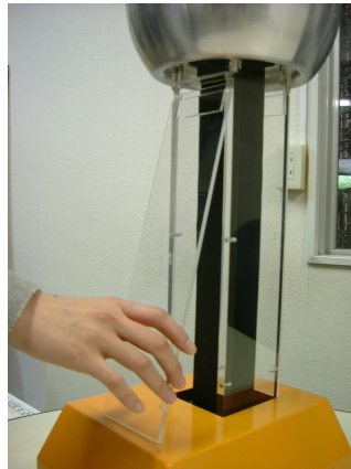
Fig. 6 Unscrewing All Screws from the Column to Remove Two Acrylic Panels
