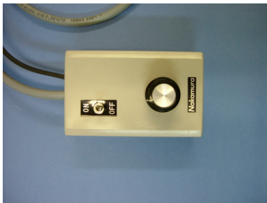
Fig. 1 Belt Speed Controller
