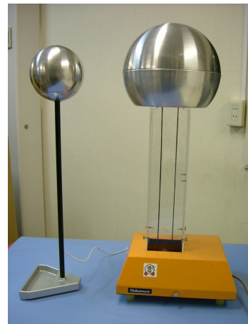
Fig. 3 Connecting the Discharge Bulb to the Raijin Main Unit
