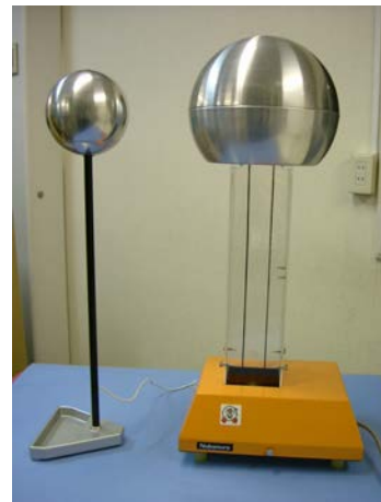
Fig. 3 Connecting the Discharge Bulb to the Raijin Main Unit
