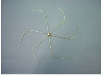
Fig. 15 Bending the Discharge Needles
