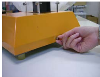
Fig. 4 Removing Screws from Lower Parts of the Side Faces of the Main Unit
