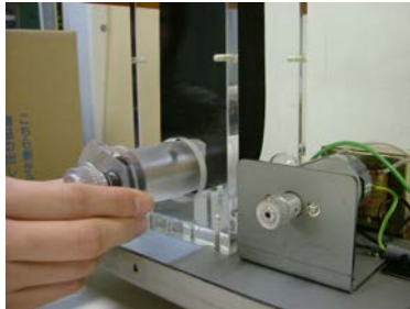
Fig. 11 Removing the Bottom Roller
