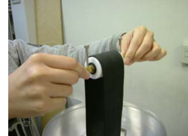
Fig. 12 Removing the Upper Roller Together with the Belt
