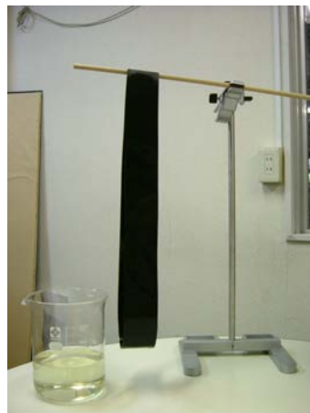
Fig. 14 Hanging the Cleaned Belt over a Pole or Rod to Dry it in the Shade in Locations with Little Dust
