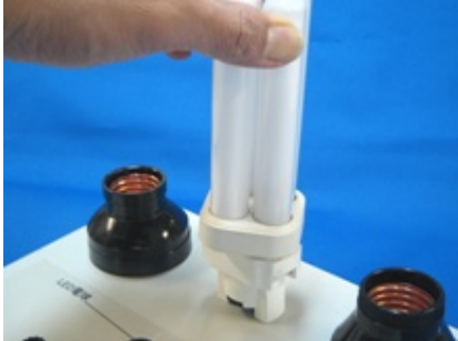
Connecting fluorescent bulb
