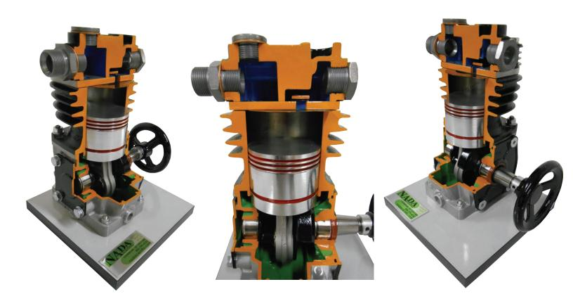
This cut-away model represents the alternative air compressor in a braking system.
