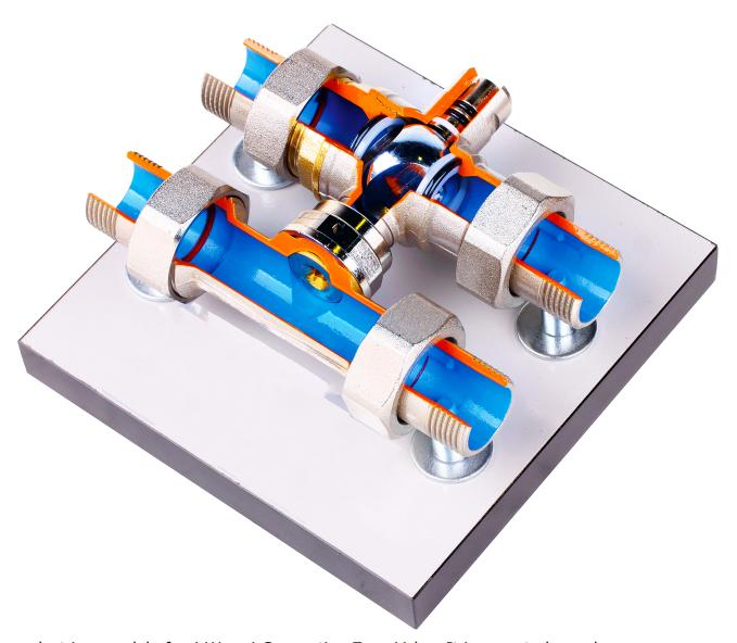
This product is a model of a 4 Way, 4 Connection Zone Valve. It is mounted on a base.
