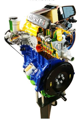
This is a 4-Cylinder Toyota Gas Engine with Variable Valve Timing with Intelligence (VVT-i), Indirect Injection. The VVT-i system varies the timing of the intake valves by adjusting the relationship between the camshaft drive and intake camshaft.
