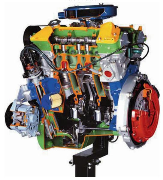
The engine operates electrically at 120 volts and runs at a reduced speed to let the student easily understand and observe the operation of the various mechanical parts.
