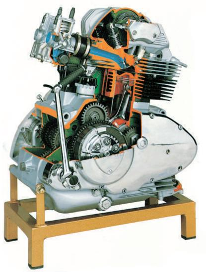
The Ducati motorcycle engine cut-away model has been carefully sectioned for training purposes, professionally painted with different colors to better differentiate the various parts, cross-sections, lubricating circuits, fuel system, cooling system, and other key components. Many parts have been chromium plated and galvanized for a longer life.
