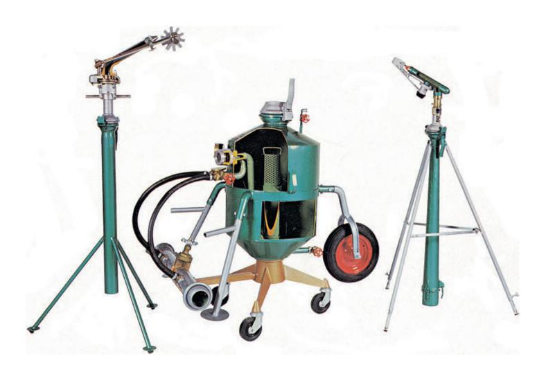
This cut-away model is comprised of a fertilizer and two irrigators of different types placed on suitable delivery pipes. The fertilizer has been fully sectioned for training purposes. Included with the unit are a pressure gauge, gate valve and rubber hoses. These features allow the real working principle of a fertilizer system to be reproduced.
