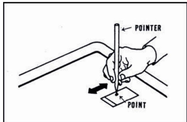
2. To operate the rotating parts, the pedal, etc. use the TRANSPARENT INSTRUCTION ROD provided. Place the rod through a pin on the part you wish to rotate, and pull or push the rod.
