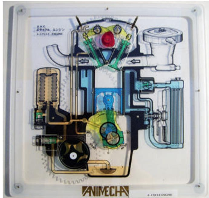
Turning the pin on this transparency will rotate the crankshaft. Students will see how the intake, compression, and exhaust processes make the engine work. On average, the engine rotates one thousand times each minute, generating a tremendous amount of heat and friction. Oil pumped through the engine coats the moving parts, reducing friction. At the same time, oil cools, cleans, and helps to seal the combustion chambers. Use the relief valve and bypass valve to understand the cooling device.
