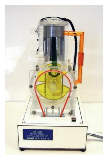
This product is a model of a 2 cycle engine. A transparent plastic housing enables students to see the internal structure at all angles.
